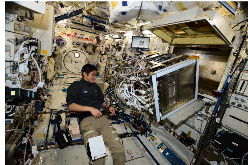
Electrostatic Levitation Furnace (ELF) attached to the Multi-purpose Small Payload Rack 2 (MSPR-2). Photo Credit: JAXA/NASA
