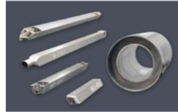
Fuel rods for nuclear propulsion. Photo Credit: NASA
