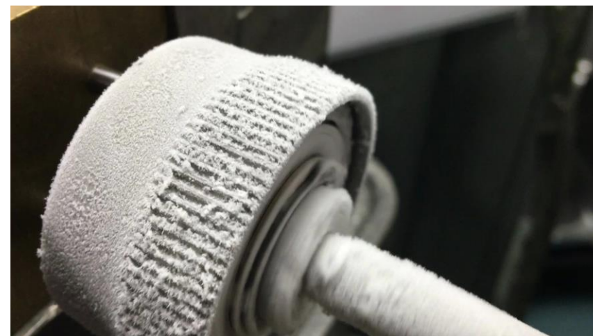
A bulk metallic glass (BMG) gear during cryogenic testing by NASA.
