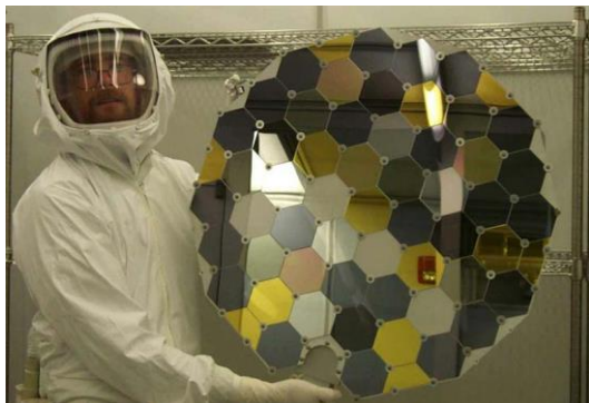
One of the solar arrays loaded with 55 detectors
