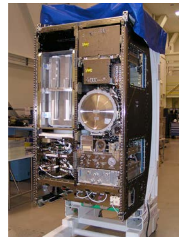
Materials Science Research Rack (MSRR) ground unit.
