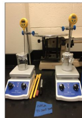
Figure 4: Image shows the dissolution setup. Left: PVDF dissolving in acetone. Right: PC dissolving in acetone
