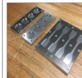
Figures 5-6: Stainless steel wafer and dog bone molds for formation of dissolutionized test samples (left). Carbon fiber reinforced ULTEM samples made using rudimentary molds (right).
