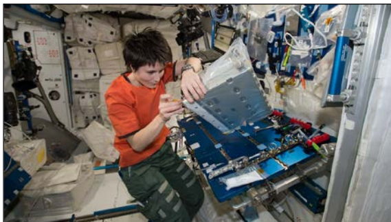
European Space Agency Astronaut Samantha Cristoforetti is shown repairing a controller panel on the ISS, a task included in the Mars expedition task lists.
