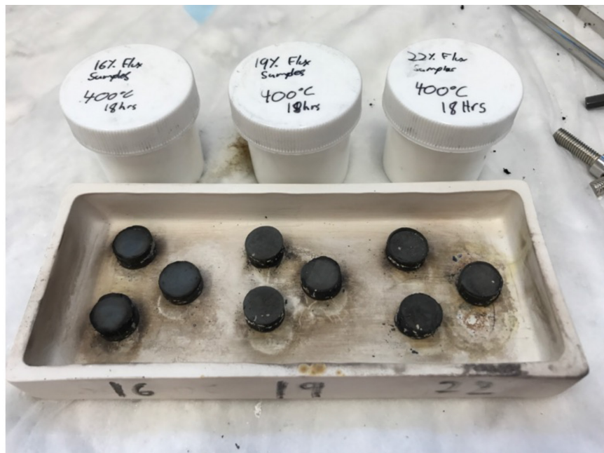
Figure 4. Ink samples sintered at 400 °C for 18 hours with labeled flux percentages of 16%, 19%, and 22%.
