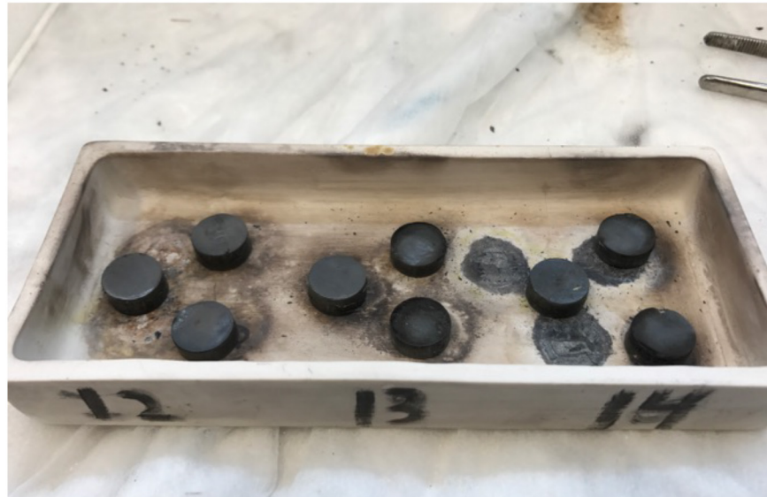
Figure 7. Samples sintered at 400 °C for 18 hours with a 12%, 13%, and 14% flux composition.
