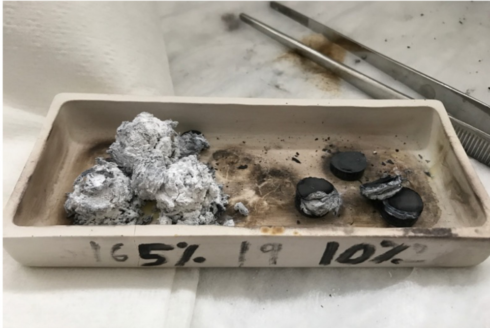
Figure 5. Ink samples sintered at 400 °C for 18 hours with labeled flux percentages of 5% and 10%.
