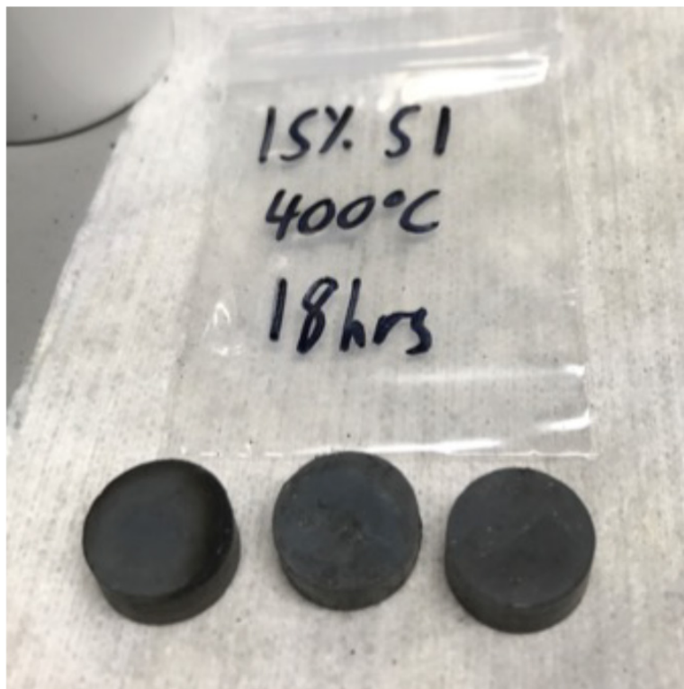
Figure 6. Samples sintered at 400 °C for 18 hours with a 15% flux composition ink.
