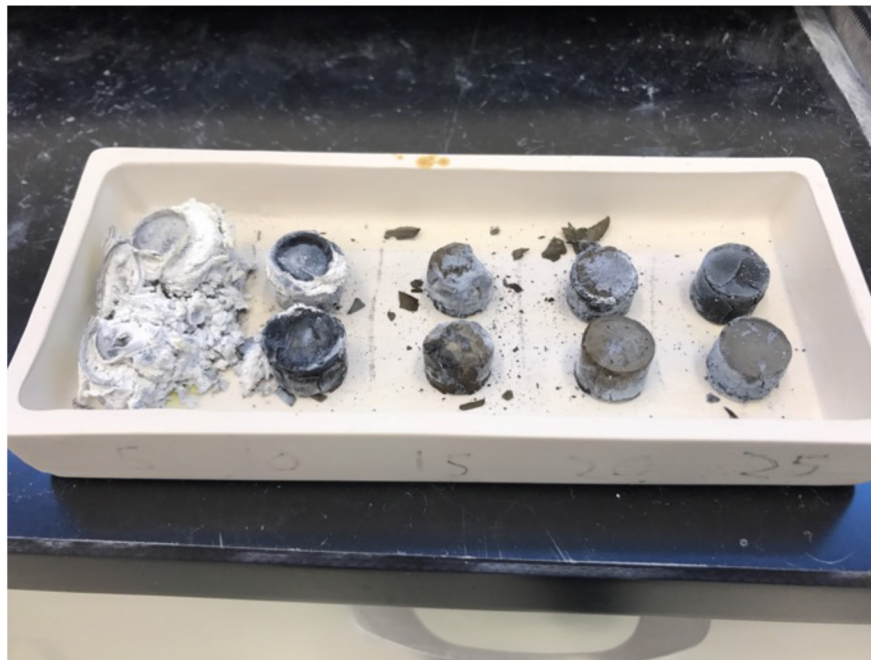
Figure 2. Ink samples sintered at 600 °C for 18 hours with flux percentages of 5%, 10%, 15%, 20%, and 25% in order from left to right (two samples at each composition).
