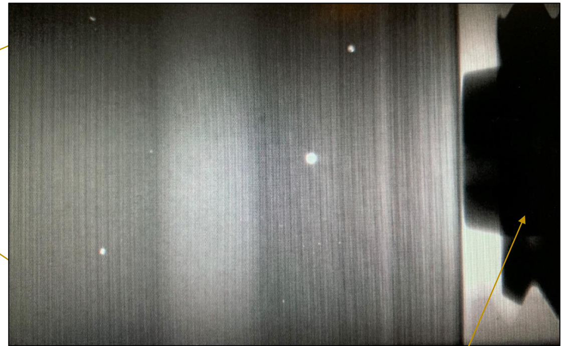
X-Ray Image: Image reveals the contact between the TC set screw assembly and an 18650 Li-ion cells installed in the FTRC during testing at Diamond Light Source in 2019.
