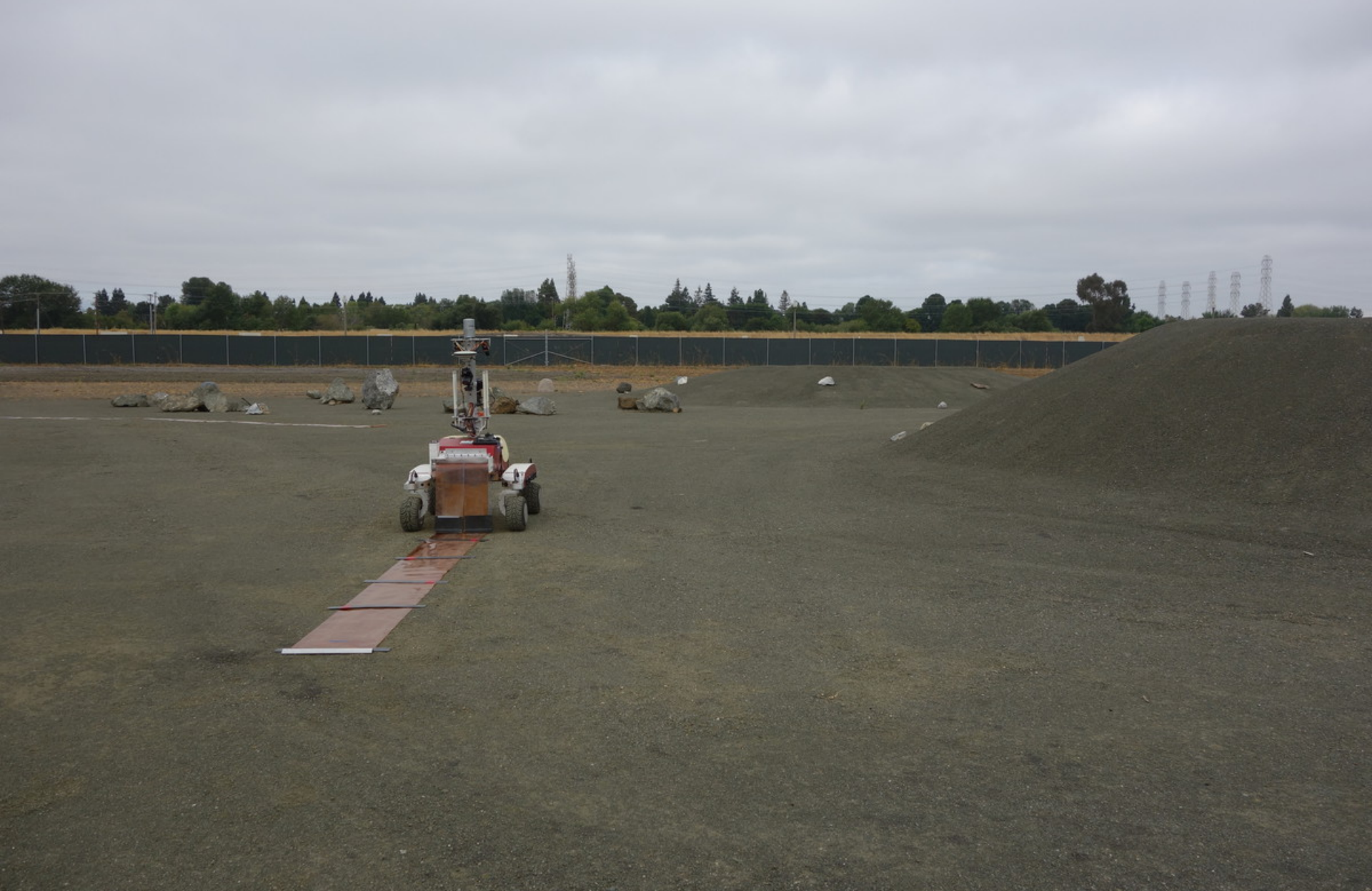
K10 deploying simulated polyimide antenna
