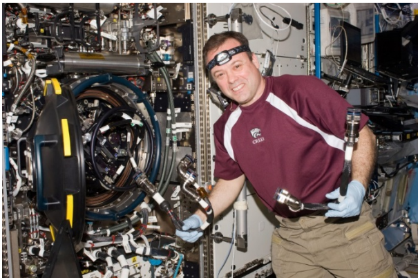
Astronaut Ron Garan configuring the Combustion Integrated Rack (CIR) for FLEX experiment
