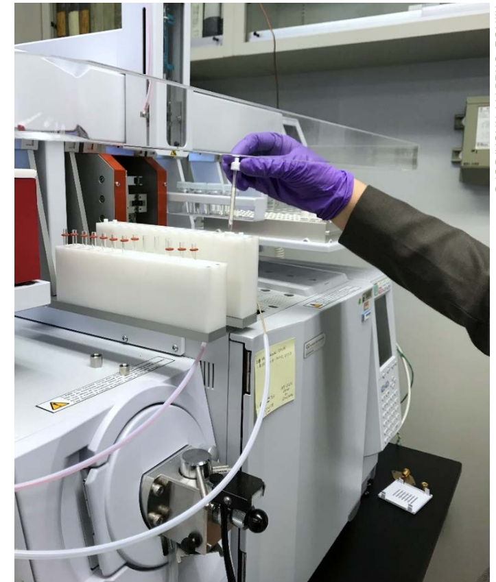
A sample tube with the released compounds is ready for placement in the sample holder on the GC/MS
