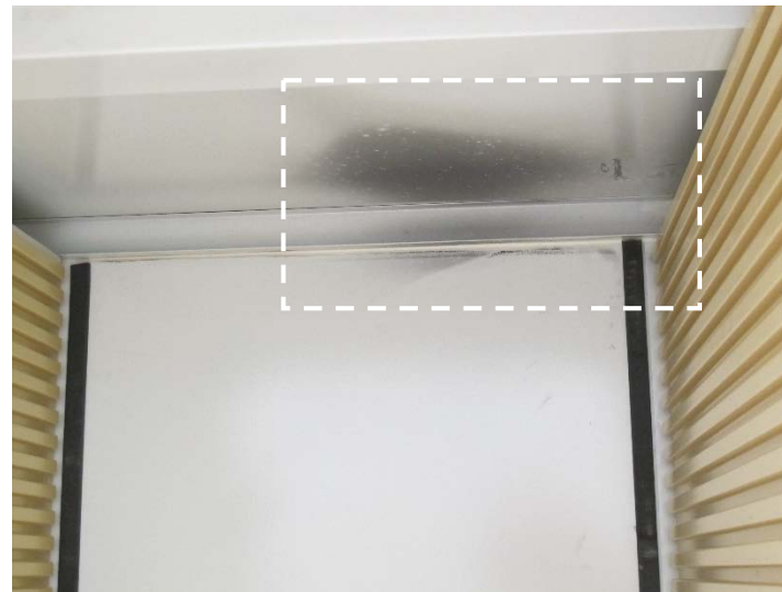
Visible dark stains of mercury contamination on cabinet surfaces
