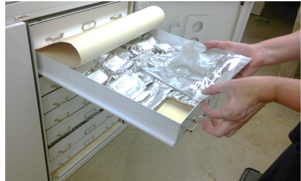
Mercury ores enclosed in vapor impermeable Marvelseal bags
