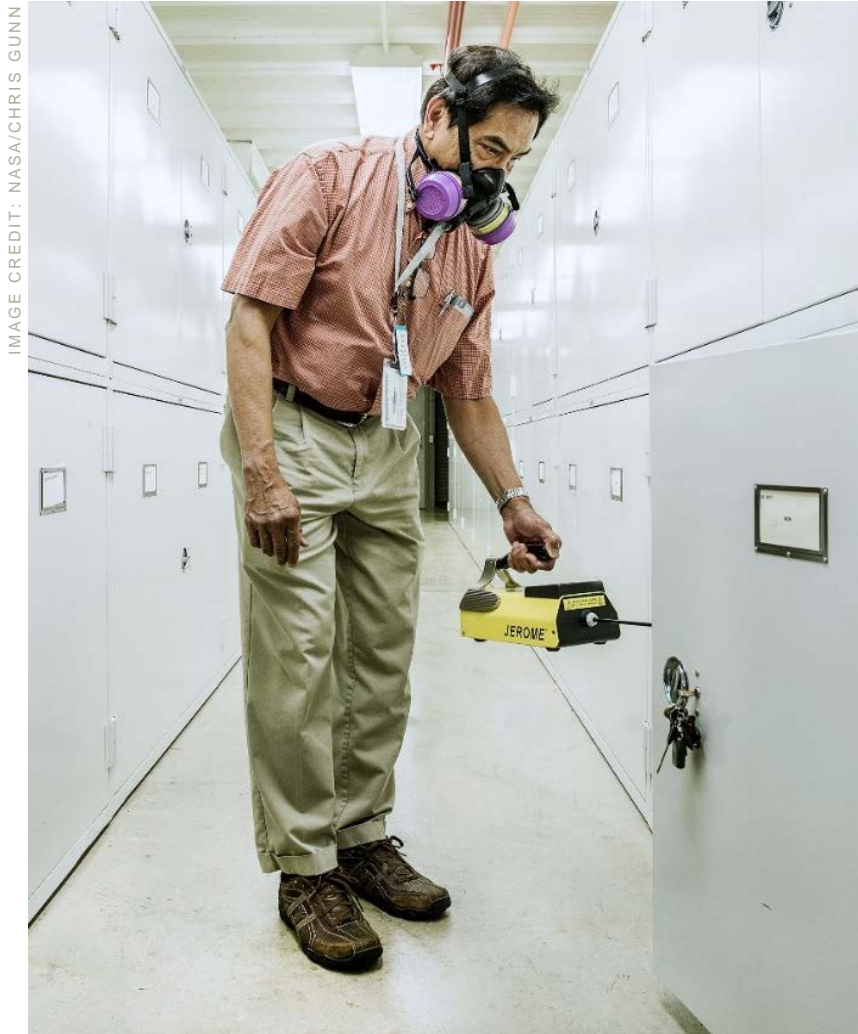
GSFC Industrial Hygienist wearing a respirator and using a Jerome mercury vapor analyzer prior to a sample retrieval effort
