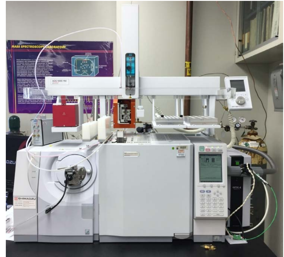
Shimadzu GC/MS QP2010 Ultra used for testing efforts at GSFC
