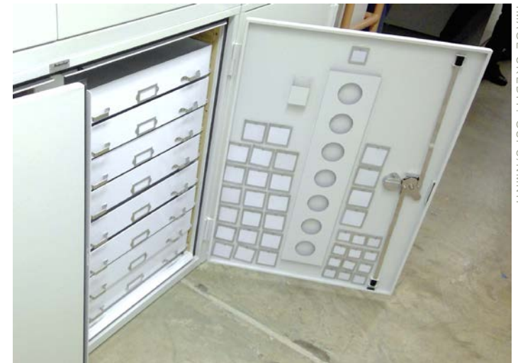
MAC samples installed in Cabinet 3 (Control) for the initial year-long experiment at MSC
