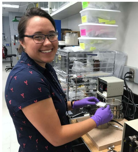
TD-GC/MS testing of a 2" by 2" MAC sample using the Scientific Instrument Services (SIS) heated thermal desorption sampling chamber
