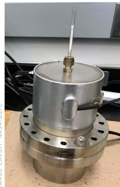
TD-GC/MS testing of a 2" by 2" MAC sample using the Scientific Instrument Services (SIS) heated thermal desorption sampling chamber
