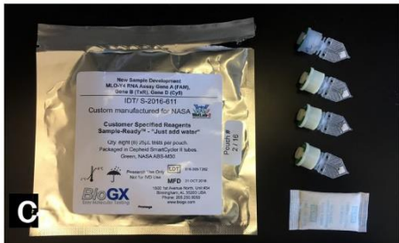
Lyophilized All-In-One Reverse Transcription of mRNAs and PCR Amplification of cDNAs or gDNA Flight Validated on ISS (Room Temperature Storage)
