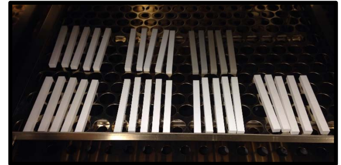
Drying Oven 100C, <5% rel. humidity, 50 days
