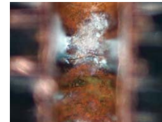
Optical micrograph of cross section of PTH with etch damage (dark field)
