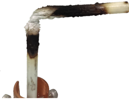
Figure 4. Sample of axially oriented GFRP inserted in argon plasma for 80 seconds (considered demised).
