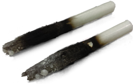
Figure 5. Sample of axially oriented GFRP inserted in air plasma until demise
