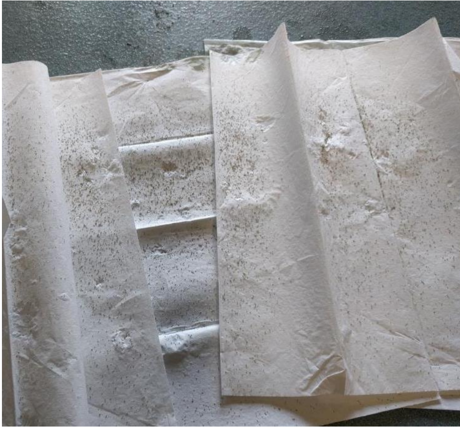
Figure 6. Flakes of contaminant removed from screen during cleaning. Lab wipes (approximately 30 cm x 30cm each) positioned below screen to facilitate clean-up.
