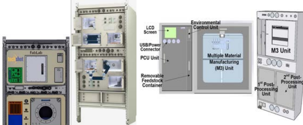
Multimaterials Fab Lab - Capable of Printing Metals and Electronics (Interlog, Techshot, Tethers Unlimited) – ISS Installation in FY22
