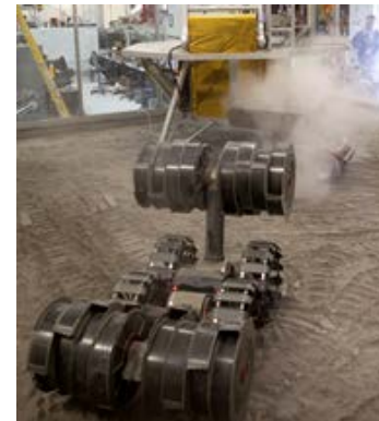
RASSOR excavator delivering regolith
