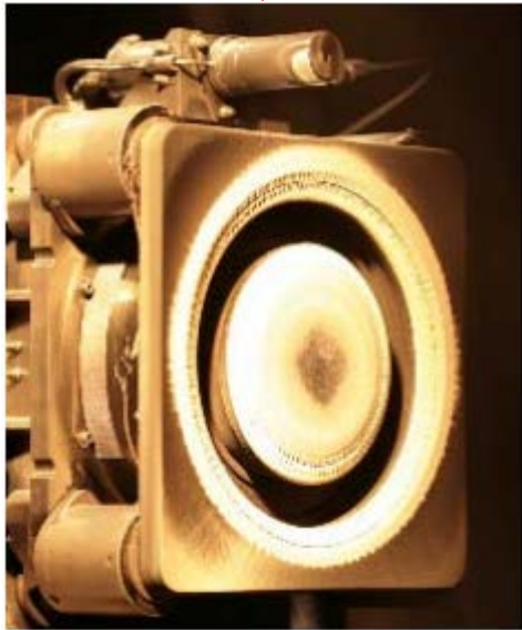
Life limited by erosion of discharge channel
