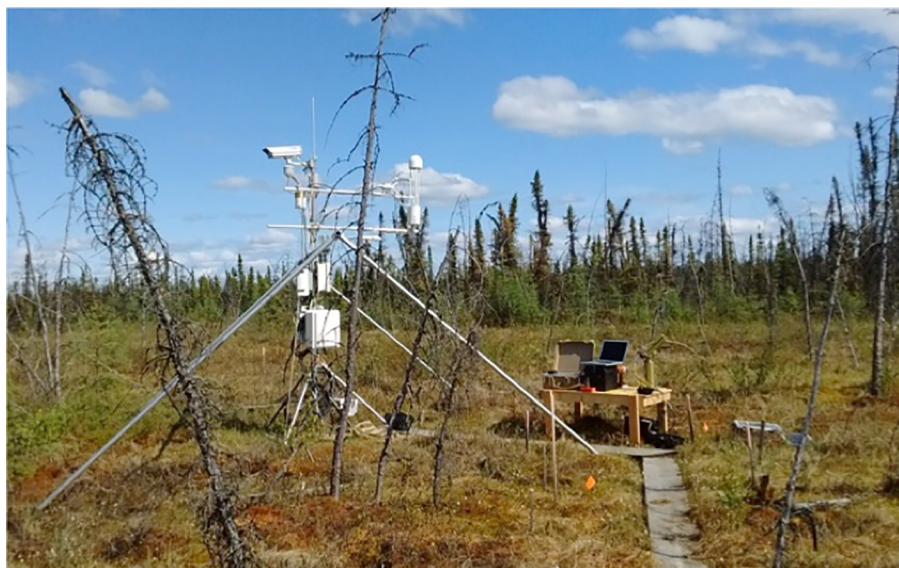
Figure 1. The mini-LHR (right) is portable and can be deployed to remote locations where larger TCCON installations are not possible due to the fragile ground conditions. Shown here are the mini-LHR monitors XCO 2 and XCH 4 alongside an eddy-covariance tower (left) in a collapse-scar bog permafrost site in Alaska.
