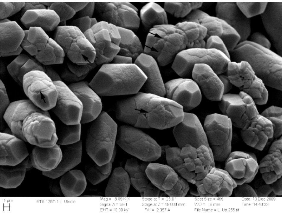
SEM image of utricular otoconia from 90-day MDS flight Mouse. Arrows indicate regions of assumed restructuring of the individual particle. [8kX magn.]
