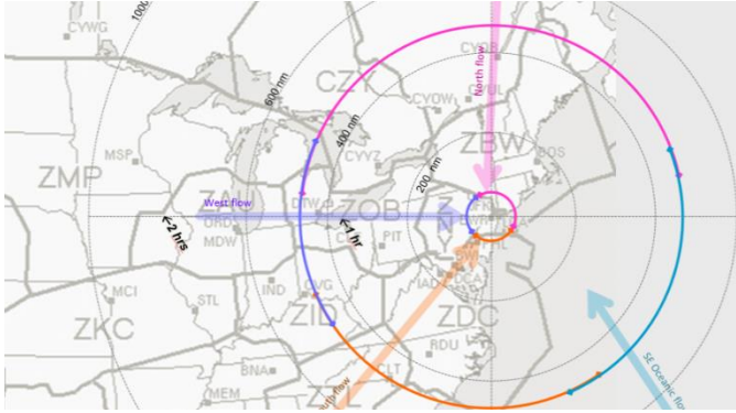
Figure 1. Schematic representation of CTOP Flow Control Arcs (FCAs): Upstream FEAs (outer arcs) and schedule to an airport (inner ring)
