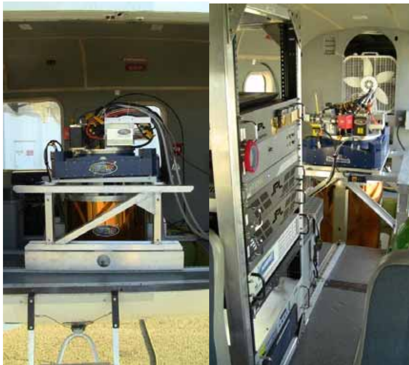
Figure 4: Side view (left) and front view (right) of JPLs AVIRIS-NG instrument installed aboard the Twin Otter International research aircraft. Right picture shows the instrument control units installed in front of the instrument. Credits: Jet Propulsion Laboratory, California Institute of Technology.
