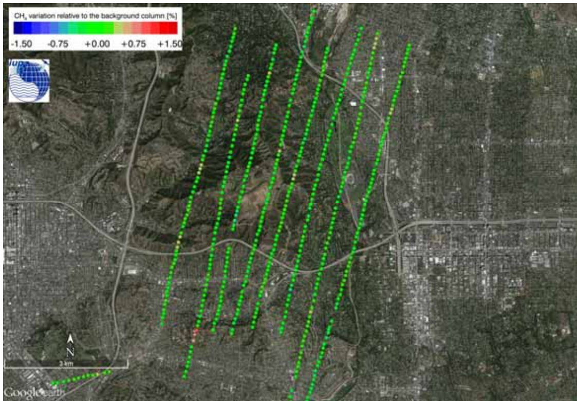
Figure 90: Normalized column averaged dry air mole fraction of CH_4 of the MAMAP remote sensing sounding of the Scholl Canyon Landfill on 2014-08-27.
