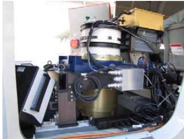
Figure 6: Mako installed in a DeHavilland DHC-6 Twin Otter aircraft.
