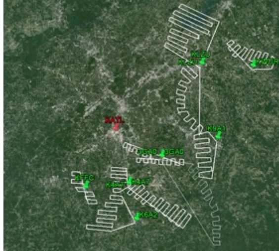
Figure 9: Stream flow monitoring missions near Atlanta, Georgia, where the green represents the departure airport and the white lines represent the UAS flight path.
