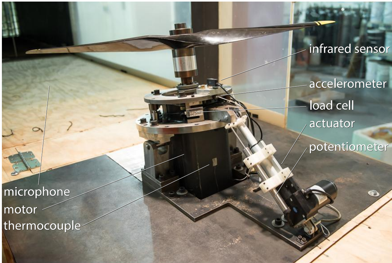
Figure 7. Hardware and sensor installation within the MARSWIT test section.
