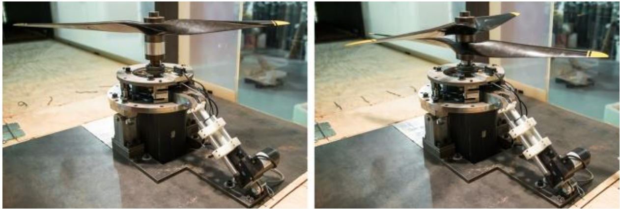
Figure 3. Left and right images show single- and dual-rotor configurations tested in the MARSWIT test section, respectively.
