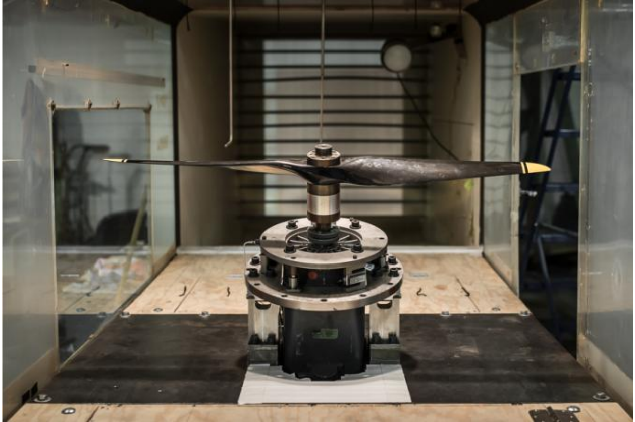
Figure 5. Single rotor at -14 -degrees shaft angle, looking downstream of the test section.
