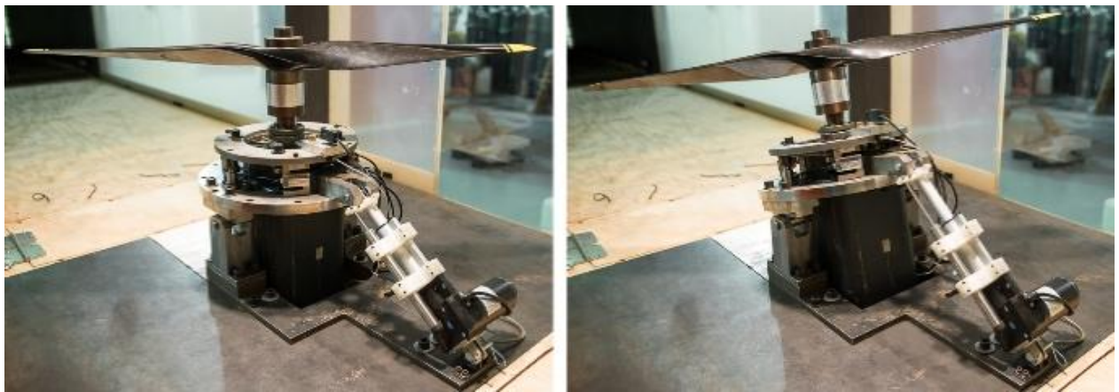
Figure 4. Left image shows single rotor at 0-degree shaft angle; right image shows single rotor at -14 -degrees shaft angle.
