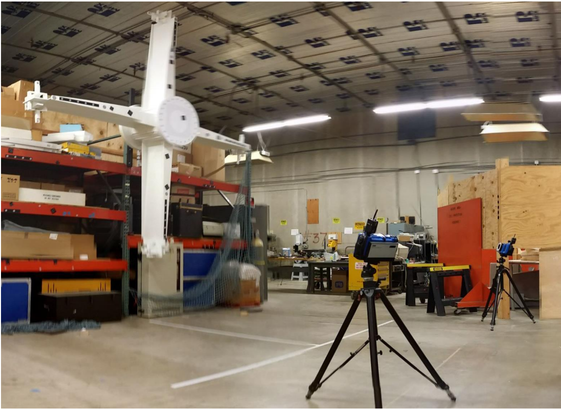
Figure 8. Bench calibration of the V-STARS/M system using a full-scale foam model of the metric hardware.
