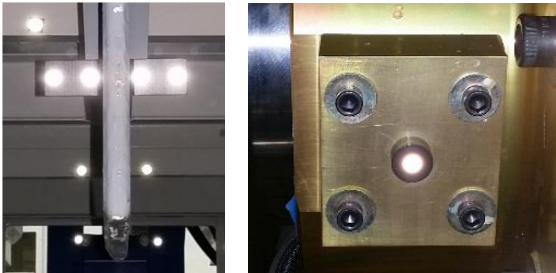
Figure 10. (Left) Roll moment linkage with custom button targets installed on each side of the moment arm. (Right) Shear block with retro-reflective button target.
