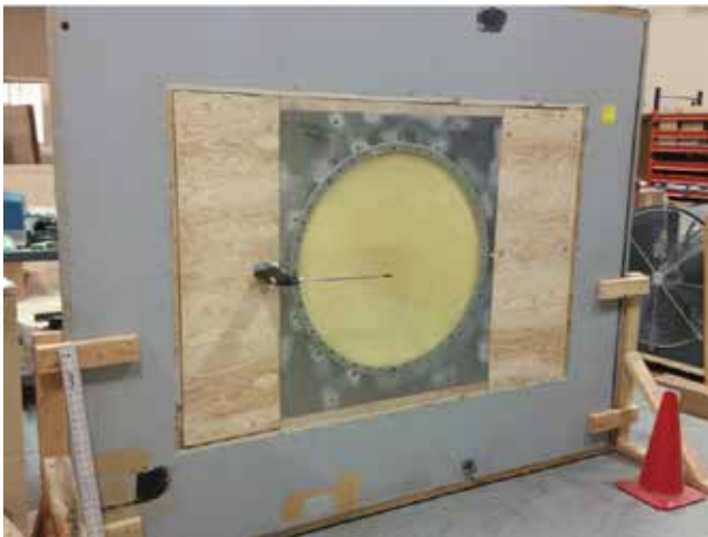
Front: Wall porous screen config
