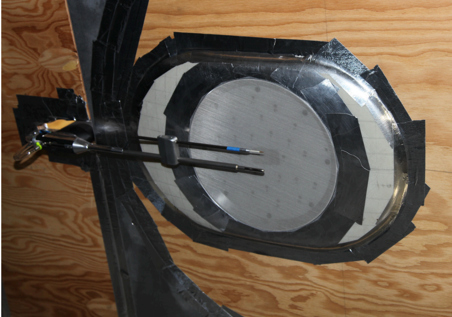
Pitot static and X-wire probe near center of wall-mounted array
