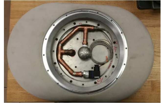
Half-airball source fairing with P and T sensors.(roam removed)
