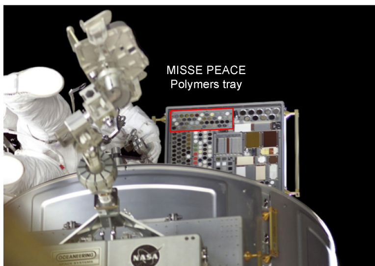
Figure 5.—Astronaut Patrick Forrester installs MISSE PEC 2 on the ISS Quest Airlock during a spacewalk on August 16, 2001.
