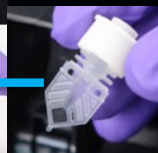
Reaction tube containing lyophilized chemical assay bead (proprietary)
