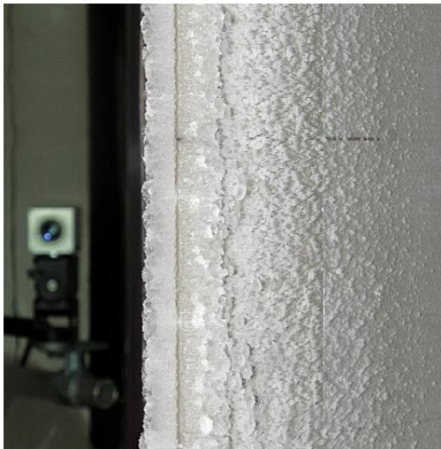
Figure 5. Photograph of leading edge ice accretion on a 21-inch chord NACA 0012 airfoil. Test number AE2741.
