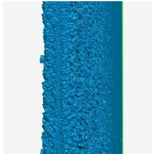
Figure 6. Scan of leading edge ice accretion on a 21-inch chord NACA 0012 airfoil. Test number AE2741.
