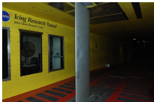
Figure 3. 21-inch chord, NACA 0012 airfoil model mounted vertically in the test section of the IRT.
