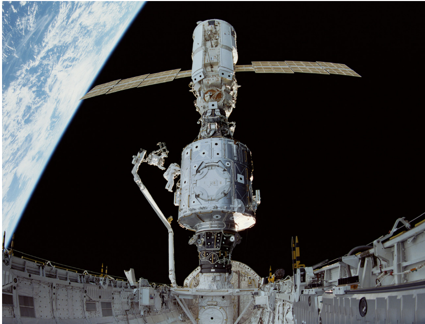
Left: Mission 2A - Zarya FGB control module – launched on a Proton rocket November 18, 1998 ( Courtesy of NASA ). Node 1 – launched on STS-88 December 6, 1998 ( Courtesy of NASA ).
