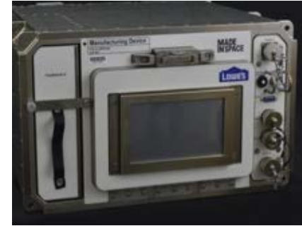
Dedicated Additive Manufacturing Facility Established on ISS – 3-D Printing Capability for NASA and Other Customers (Made in Space – 2016)
