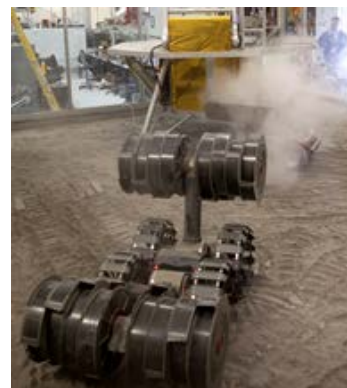
RASSOR excavator delivering regolith
