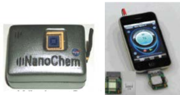
(L) CNT "Electronic Nose"; (R) Nanochemsensor flown on ISS
