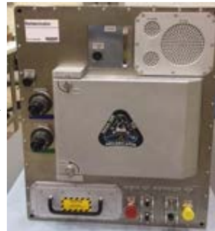
Refabricator (Integrated Recycler/3-D Printer) Installed and Activated on ISS (Tethers Unlimited – 2019)
