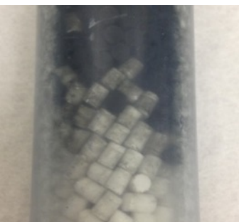
Sabatier catalyst material after vibration testing
