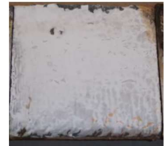
Durable slurry-coated test article after 15 hours at 2500 / 2600 / 2700°F
