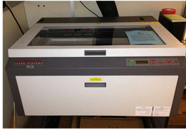
Universal Laser System (Two 60 watt laser heads and a work area of 32"x18")
