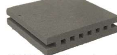
AM SiC with 1.5 mm channels
