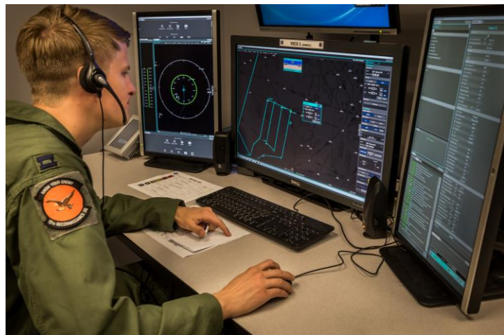
Figure 3. VSCS in Standalone configuration. TSD, bottom-center display; health and status panel, right display; Standalone DAA display, left display.
