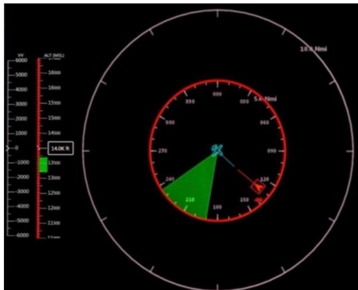
Figure 5. Screenshot of vertical and horizontal DAA maneuver guidance to regain well clear on the VSCS Standalone DAA display. The typical heading and altitude bands are fully saturated red. The two green ‘wedges’ indicate the heading and altitude options that will maximize separation with the offending aircraft.
