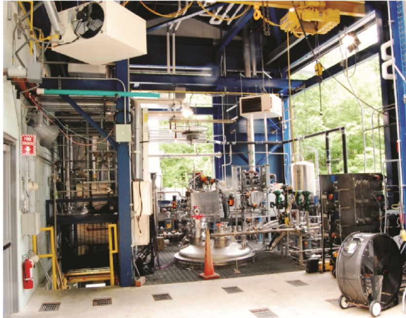
Figure 8.—The Small Multipurpose Research Facility. Core test rig, fluids system, and fluid temperature control systems will be located on floor in front.
