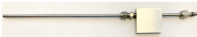
Fig. 4 1/4-inch-OD ITP with 12 inch sense line, but without installed Kulite® and coil
