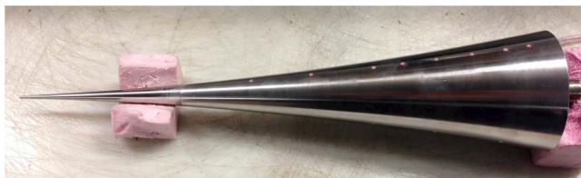
Fig. 5 Photograph of the 3-m-circular-arc flared cone.
