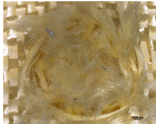
Untreated Weave Impact velocity: 2350 ft/s (Back)
