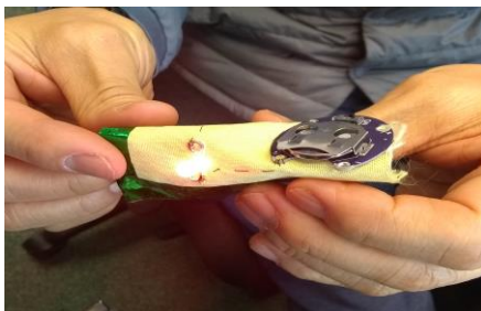
CNT yarn stitched circuit on ballistic Kevlar
