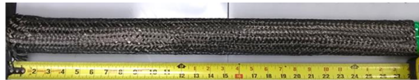
28" long Carbon fiber – CNT Yarn Hybrid Triaxial Braided Tube
