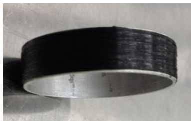
Autoclave-cured CNT overwrap
