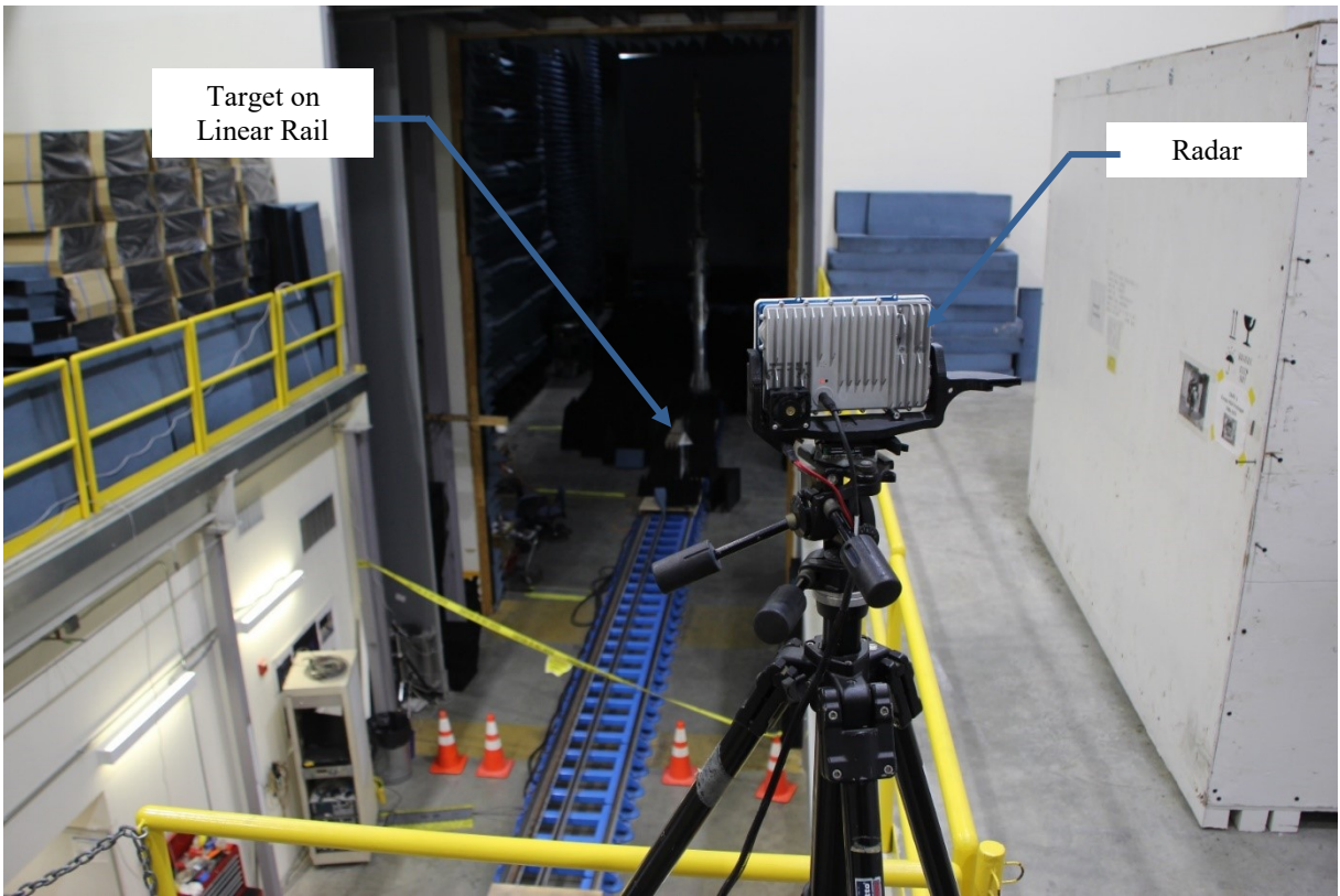
(c) View from radar of indoor test setup toward linear rail. Figure 3. Continued.
