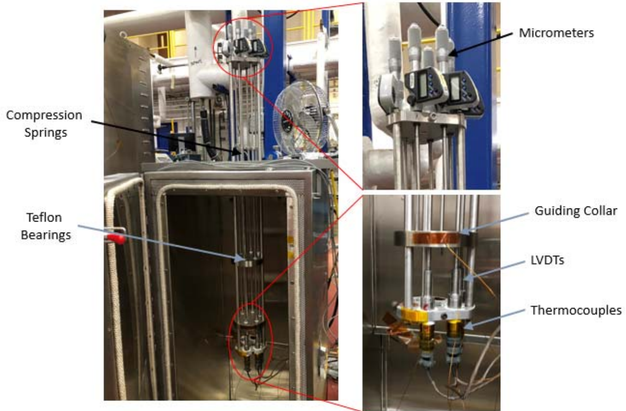
Figure 5. LVDT Calibration System.
