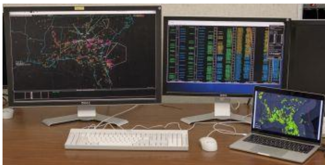
Figure 4. TMC station. PGUI on the left monitor, and TGUI on the right. Weather radar images are animated on the laptop-computer monitor.
