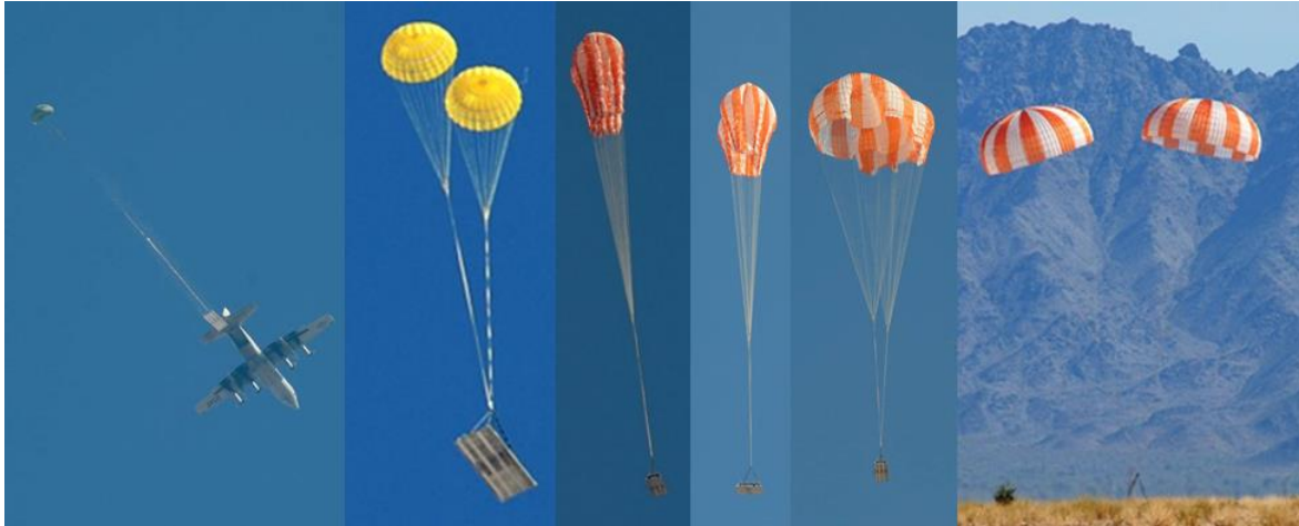
Fig. 13 Example 20ft Platform / 16ft Weight Tub Test Vehicle Test Sequence: C-130 extraction, Drogue steady state, Main first stage, Main second stage, Main full open, landing
