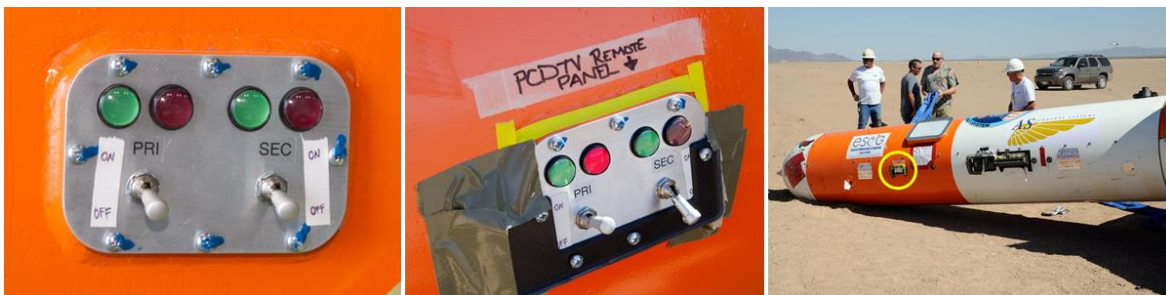
Fig. 46 CDT 3-1 Avionics Control Panel – Left to right: Both Strings Off (Down) in the Hangar; One String On (Up) and One String Off (Down) on the Drop Zone; Control Panel Location
