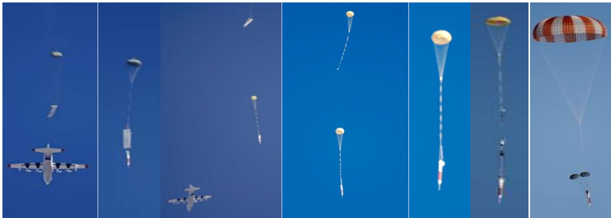
Fig. 8 Example of LVAD Medium Drop Test Vehicle Test Sequence: C-130 extraction, M-DTV/CMS separation, Programmer deploy, Drogue deploy, Drogue steady state, Main deploy, Main steady state
