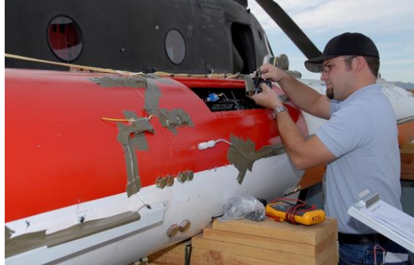
Fig. 3 Avionics Access for Small Drop Test Vehicle
