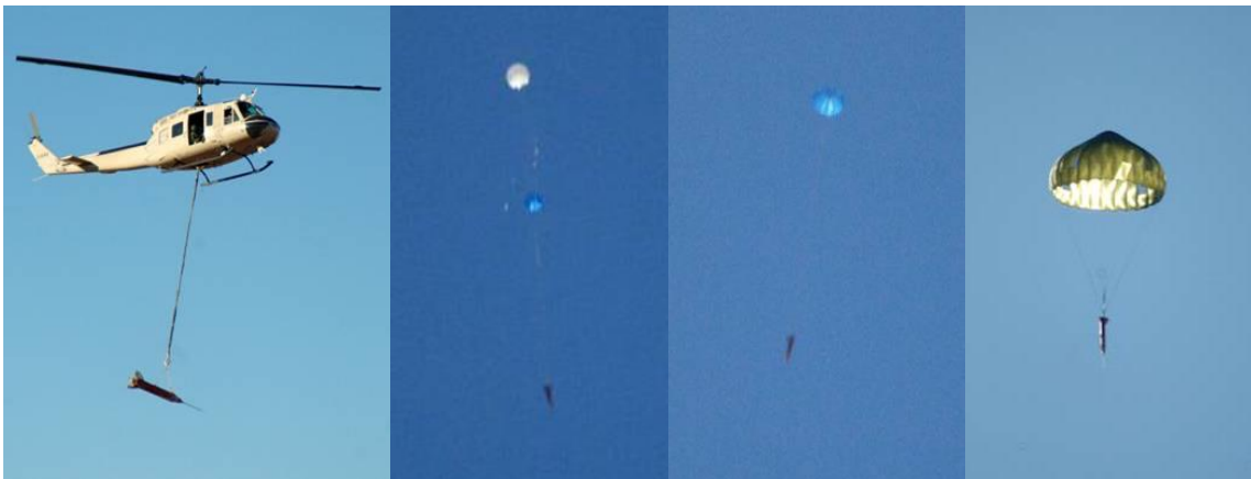
Fig. 4 Small Drop Test Vehicle Test Sequence: helicopter carry, Programmer release, Pilot steady state, Recovery parachute
