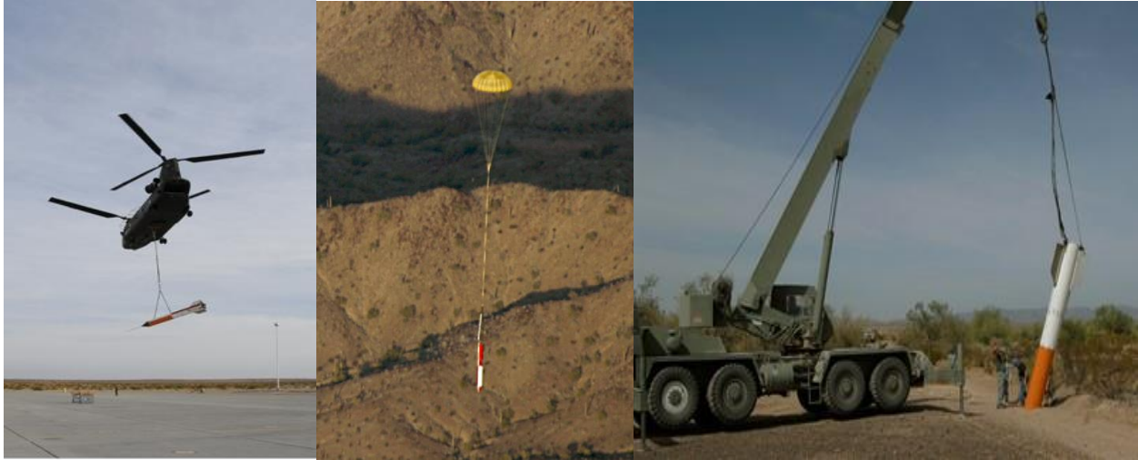
Fig. 5 Medium Drop Test Vehicle Test Sequence: helicopter carry, Drogue steady state, M-DTV recovery
