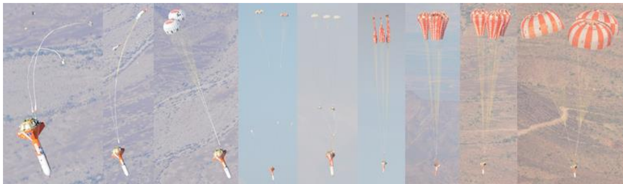
Fig. 24 Nominal (no FBCP) PCDTV Parachute Sequence: Drogue mortar fire, Drogue line stretch, Drogue release, Pilot mortar fire, Main bag lift, Main line stretch, Main first stage, Main full open
