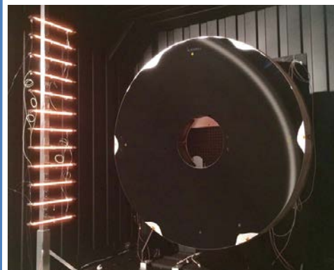
Testing surface shape response of 1.5m ULE mirror to thermal lamp array inside X-Ray & Cryogenic Facility (XRCF)
