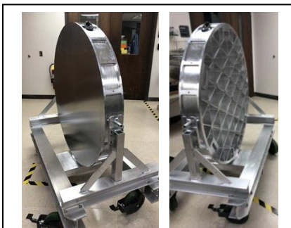
Figure 2: 1.2-m Al Test Mirror
