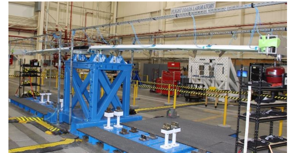
Example: Cruise Prop/Hub GVT on Foam Soft Support
