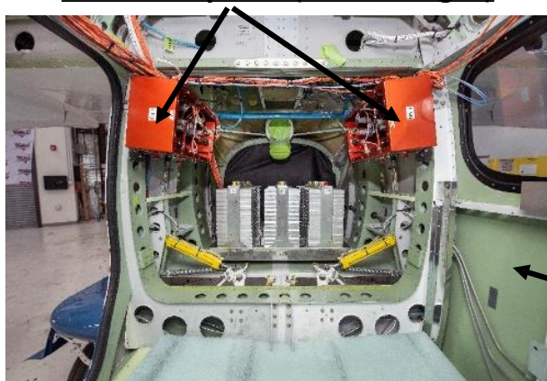
Contactor pallet (left and right)
