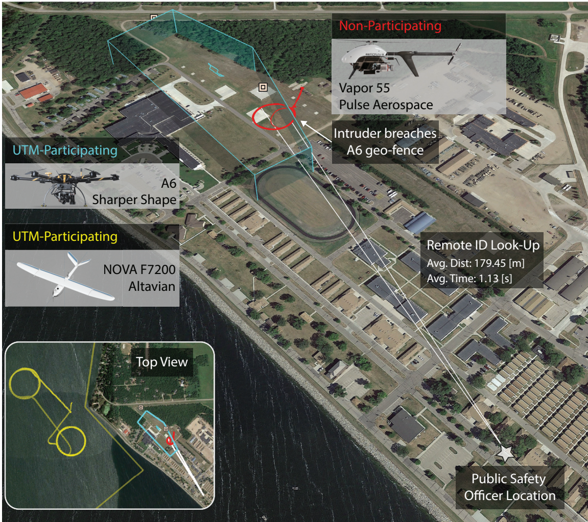
Fig. 6 Remote ID Look-Up Test: The blue trajectory depicts the A6 (participating multi-rotor) simulating a scenario of filming a sporting event. Also depicted in blue is its geo-fence. The Vapor (intruder helicopter), depicted in red, takes off and breaches the geo-fence of the A6. The public safety officer becomes aware of the intruder and uses its VID to identify the intruding vehicle. Two look-ups are shown by the white lines indicating the positions of both vehicle and public safety officer at the times of look-up. The average distance 179.45 [m] and time 1.13 [s] are computed over all data from the ND test site. Also shown is the Nova (participating fixed-wing) in yellow.
