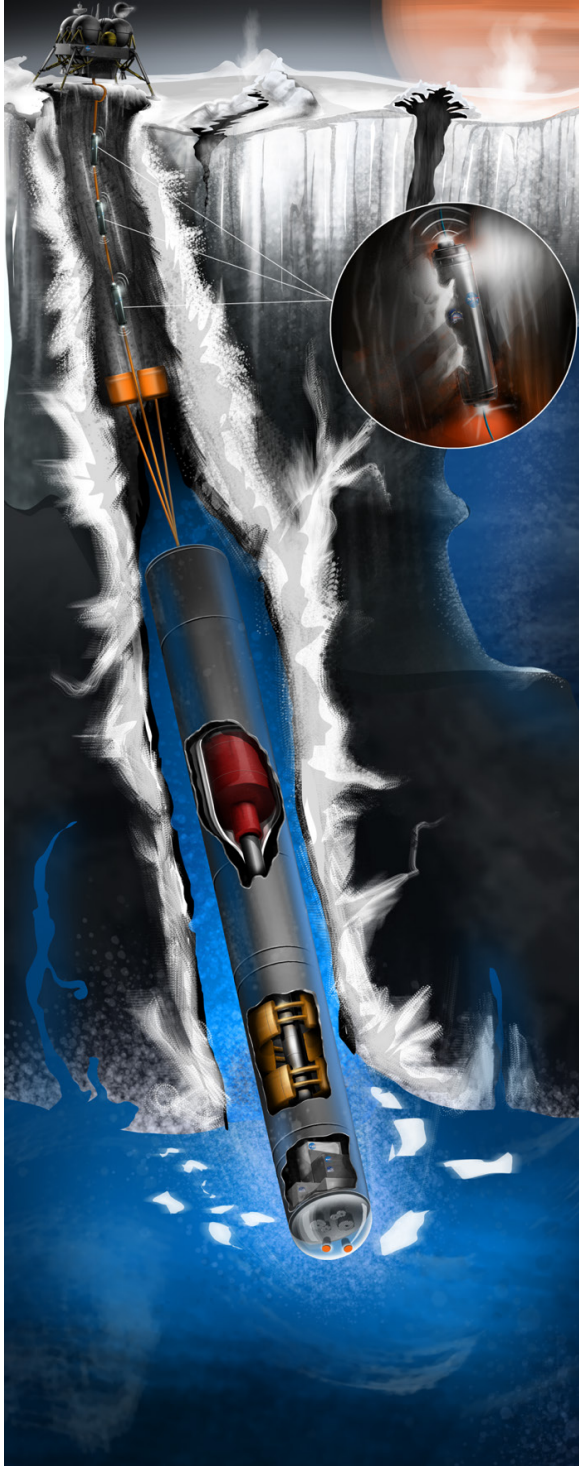
Figure 1.—Tunnelbot reaching ocean after deploying communication repeaters and anchor (artist impression).
