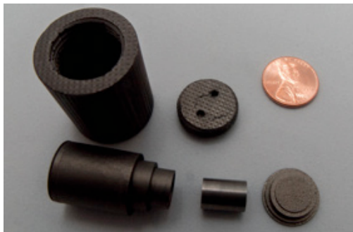
Figure 37.—Lightweight radioisotope heater unit.
