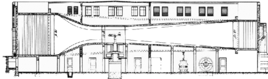
West Side View of Kirsten Wind Tunnel
