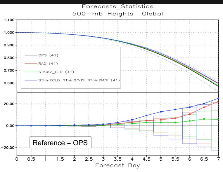
A comprehensive, adaptive thinning approach for all hyperspectral infrared sensors, using cloudcleared AIRS radiances, results in a statistically significant improvement in global forecast skill
