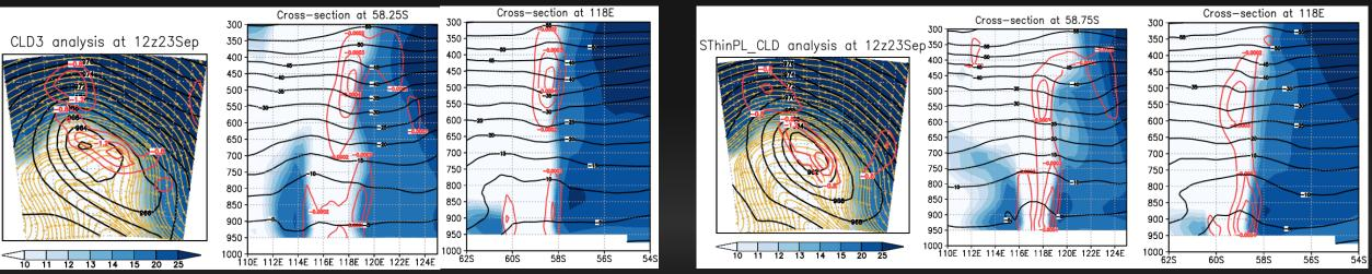
Maximum vertically integrated cyclonic vorticity and a vertically aligned eyelike feature occur when adaptively thinned AIRS CCRs are used around a polar low
