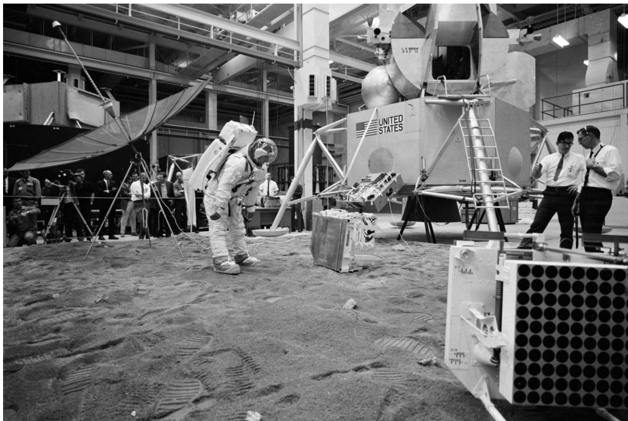
Figure 8. Test subject in the Building 9 test facilities at the Manned Spacecraft Center simulating the unpacking and setting up of some of the lunar surface instruments. (NASA photo S69-18998)
