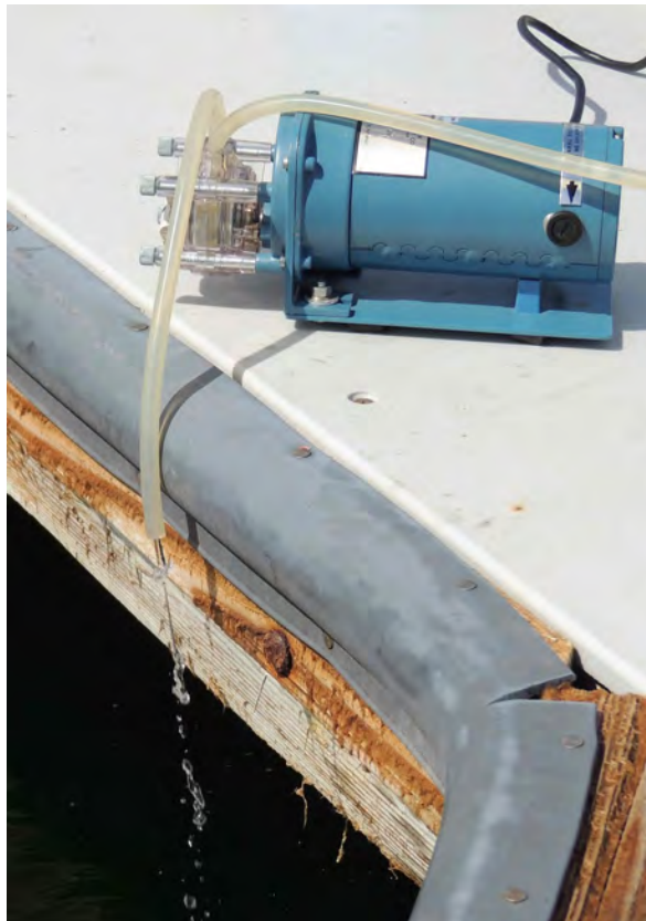
Fig. 62. The peristaltic pump, used to obtain water samples as part of the C-PUMPS accessory, in operation on a dock.
