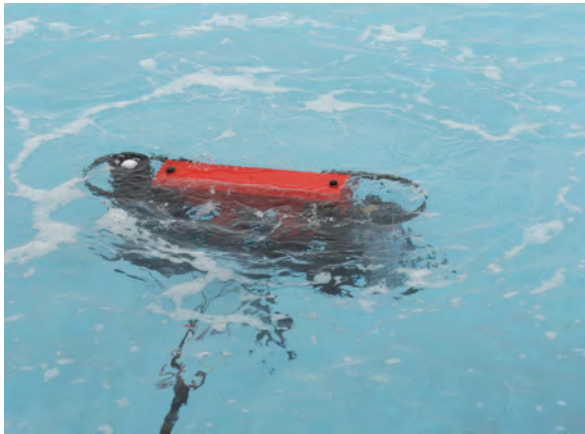
Fig. 10. The C-OPS backplane in the dissipating propeller turbulence of a small vessel reveals the large amount of bubbles formed as a result of using the propeller to push the profiler away from the boat.
