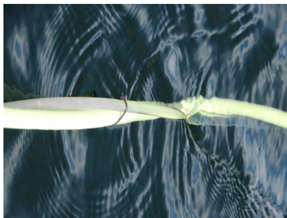
Fig. 61. The C-PUMPS tubing attached to the light green C-OPS sea cable with black cable ties.
