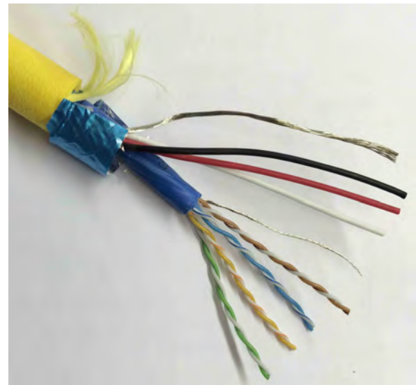
Fig. 28. The C-HyR cable with outer foam jacket (bright yellow) stripped back to reveal the strength members (pale yellow Kevlar fibers), shields (e.g., blue foil folded back over the foam jacket), drain wires (bare silver), and power conductors (white, red, and black), plus the twisted-pair conductors.
