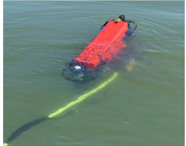
Fig. 22. C-OPS deployed in Mono Lake (California) and being maneuvered with C-PrOPS, wherein the radiance end cap is propelled above the surface and the irradiance aperture is pulled below (the irradiance diffuser is visible as the white disc immediately between the green sea cable and the red hydrobaric flotation chamber).
