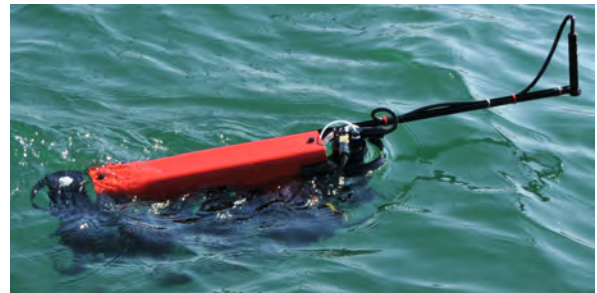
Fig. 25. The C-HyR prototype being propelled by C-PrOPS thrusters, wherein the white disk of the E_d aperture (left) is pushed down below the water surface, and the single-channel MML-100 L_u aperture at the end of the RCA (right) is raised above the water surface.
