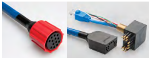
Fig. 27. A SubConn DIL13F (left) circular connector next to a DLPBH13M bulkhead (right) with mating DLPIL13F connector (left of right). The strap that holds the mated DLP connectors together is not shown, but the DIL red locking sleeve is shown.
