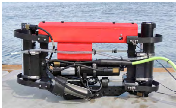
Fig. 60. The C-OPS radiometers (left and right) with the C-PrOPS and C-PUMPS accessories fitted to the backplane. The clear hose for the latter is attached to the light green sea cable and then strung right to left across the middle of the backplane.
