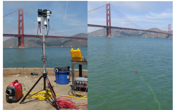
Fig. 24. The deployment of a C-OPS using the C-PrOPS and C-CAPS accessories from Torpedo Wharf near the Golden Gate Bridge in San Francisco Bay, wherein the reference and support equipment (left) are shown with the profiler (right).
