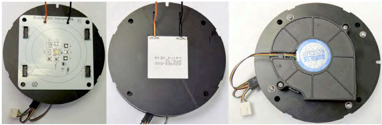
Fig. 133. The CQM MCPCB with electrical connectors on the outer rim and LED array in the center (left), which is mounted to a heat sink plus TEC within a cavity (middle), and the entire assembly is cooled with a digitally controlled fan (right). The images have different scales to distinguish different features.
