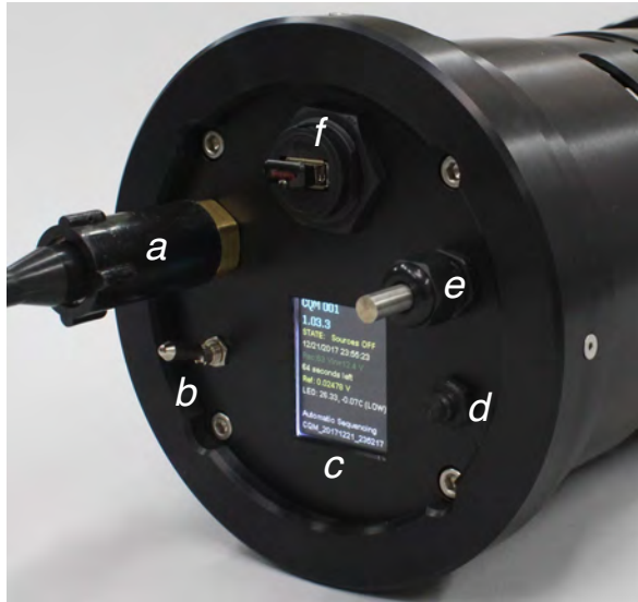
Fig. 137. The CQM backplate showing the following: a) bulkhead connector, b) power switch, c) LCD, d) mode select button, e) ambient temperature sensor, and f) USB flash memory port.
