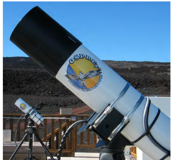
Fig. 117. An OSPRey dyad making measurements at the Mauna Loa Observatory (MLO). The foreground radiometer is equipped with a removable shroud and the background instrument has no shroud (the solar references are not visible).
