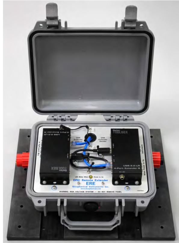
Fig. 111. The ERE as an assembled unit with mounting plate affixed to the bottom of the waterproof case, which is removable.
