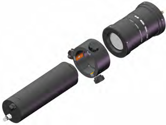
Fig. 140. The three main components for a CERT session: the DUT (left), the kinematic collar (middle), and the CQM (right). The precision DC external power supply for the CQM is not shown.
