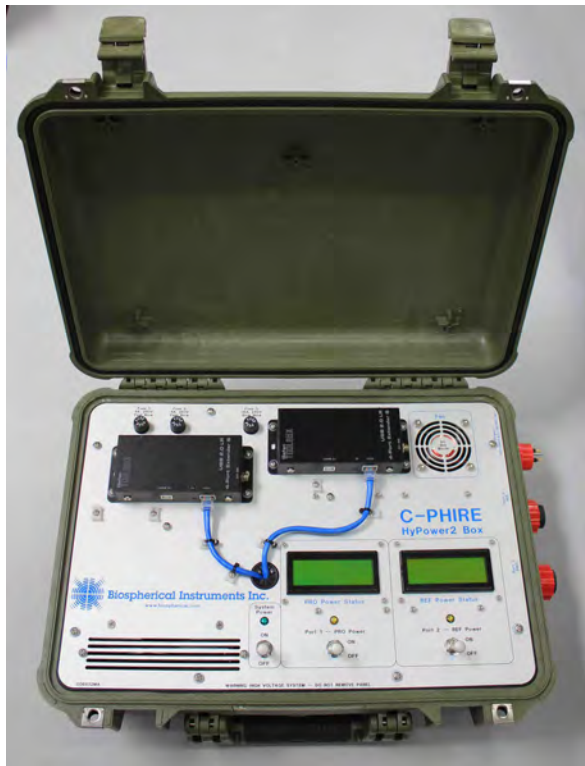
Fig. 113. The HyPower2 box showing the two USB extenders (black with blue cables) and the displays (green) for the two cable ports (red, wherein one is for AC power).
