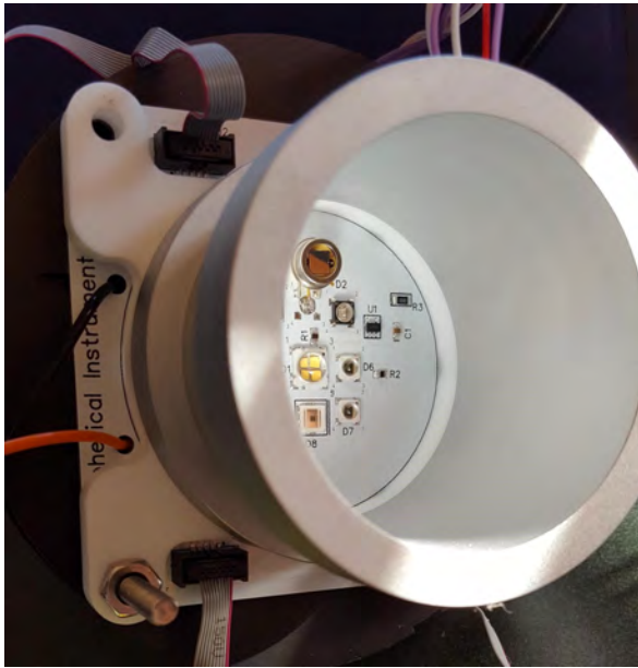
Fig. 135. The CQM light chamber showing the bead-blasted aluminum interior walls and a portion of the MCPCB.
