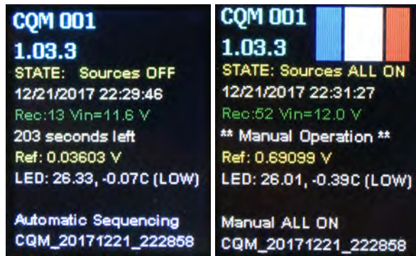
Fig. 138. The LCD indicating the status of a variety of CQM parameters for automatic and manual operational modes (left and right, respectively).
